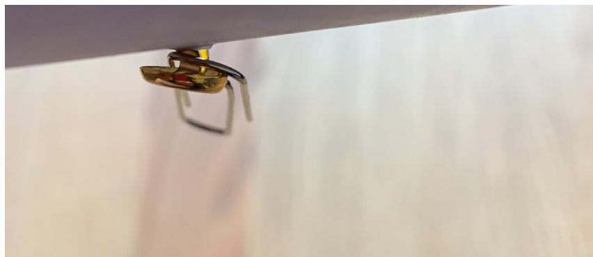
Figure 2.4: If the paper fastener is too tight, the paper clip will not spin.
